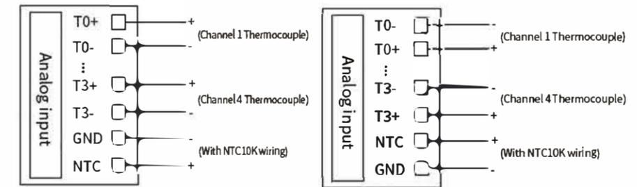
Figure 14 Customized 43C thermocouple wiring
