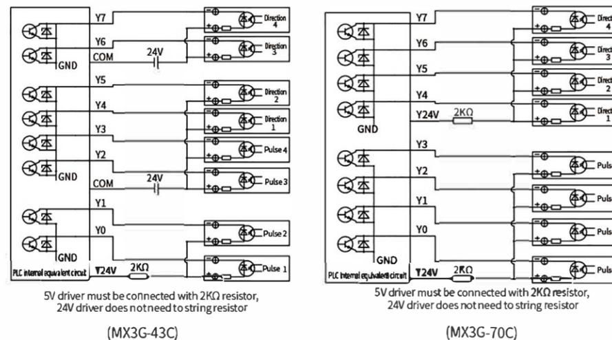
5V driver must be connected with 2kΩ resistor, 24V driver does not need to string resistor
