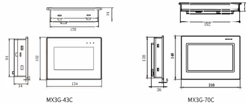
Figure 1 Installation dimension
