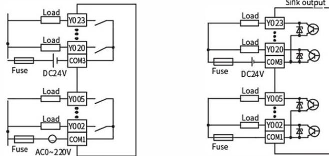
Figure 8 Relay output equivalent circuit
